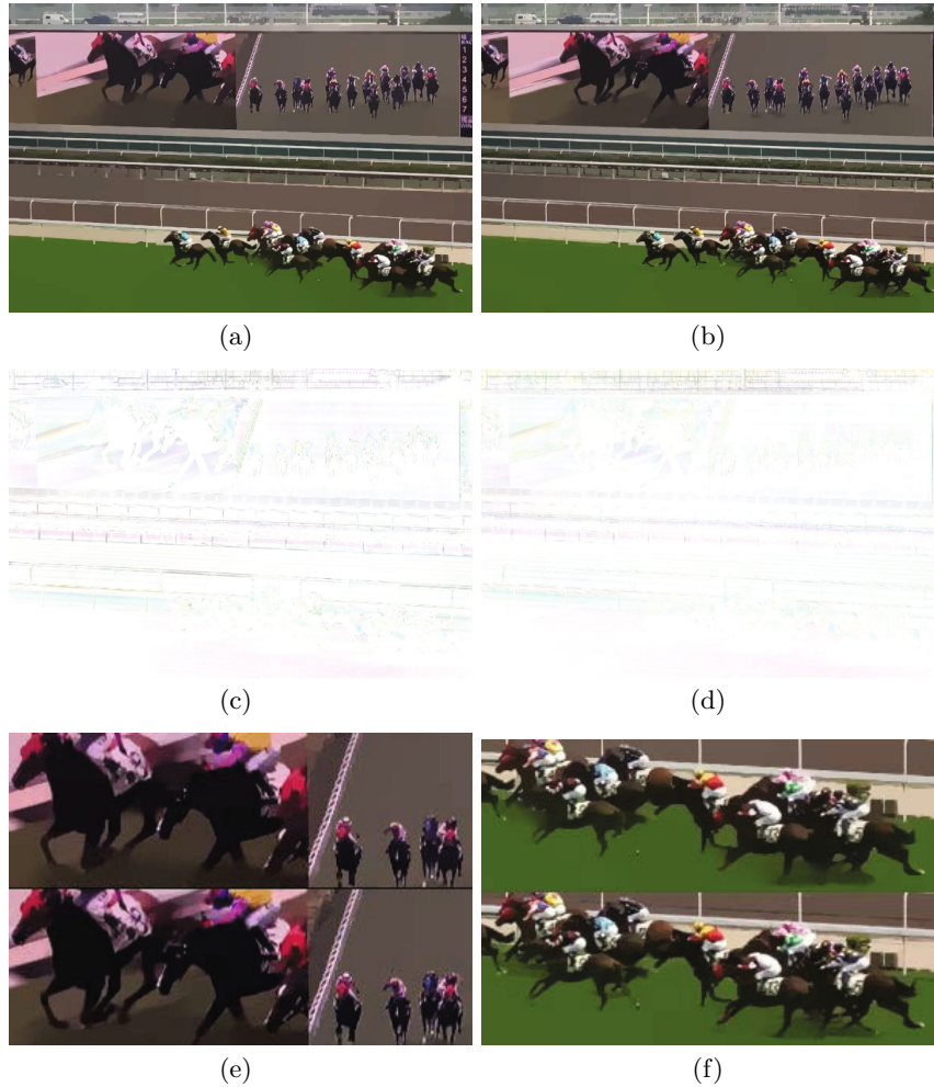
Fig. 2. Comparison of the decomposed results. To better appreciate the difference, the negative images of the detail images are given. Input image courtesy of Li Xu. (a) Smoothing layer obtained by the scheme in [3]. (b) Smoothing layer obtained by the proposed scheme. (c) Detail layer obtained by the scheme in [3]. (d) Detail layer obtained by the proposed scheme. (e) Closeups of (a) and (b). (f) Closeups of (a) and (b).
